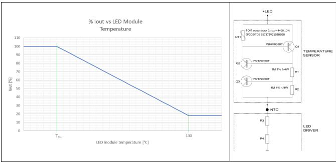
The thermal measurement is performed connecting NTC circuit from the pin LED+ and the NTC pin.
