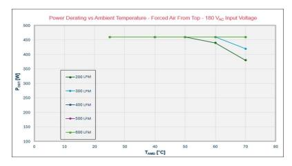
The above curves come from a climatic static chamber and a specific set up therefore they represent a thermal performance approximation of a DDP520 installed into a system where not all the variables can be controlled. Although they are a reasonable reference, it is always a recommended practice to monitor the power supply critical components temperature when operating into a system (see below hot-spots thermal map).
