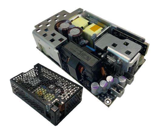
Coming in a 3 x 5" open frame package, it offers a 520 W long lasting peak power, a layout optimized for free-air-cooling environments and a universal  $90 - 305 \, V_{AC}$  input operating voltage range.
