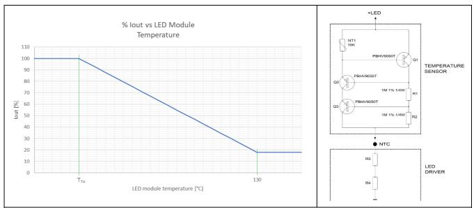
The thermal measurement is performed connecting NTC circuit from the pin LED+ and the NTC pin.
