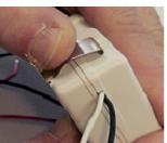
2. Rotate the upper part of the clip up towards the larger indentation on the top of the driver.
