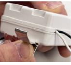
**3**. With a finger at the base of the clip, apply gentle pressure upward on the clip.
